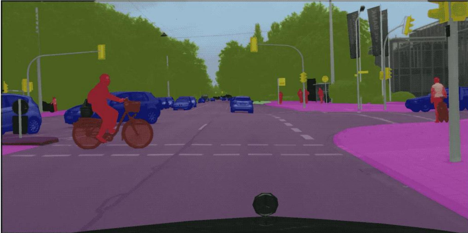
The self-driving algorithms will segment pedestrians, other vehicles, lanes, sidewalks, traffic signs, houses, grass, trees, etc. in the image according to their categories, so as to assist the vehicle to perceive the road situation
